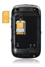
Slide the SIM card into the slot.
