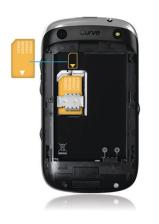
Slide the SIM card into the slot.
