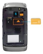
Slide the SIM card into the slot.
