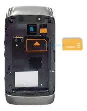
Slide the SIM card into the slot.
