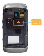
Slide the SIM card into the slot.
