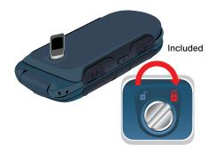
Use the battery cover removal tool to turn the dial clockwise until the cover is locked.
