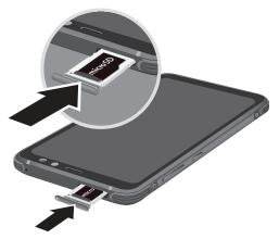
5. Slide the SIM card/Memory card tray back into the slot.
