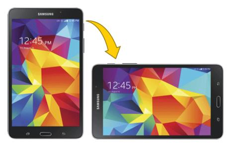
**Note**: Screen rotation needs to be enabled for the screen orientation to automatically change. Touch and drag down the notification panel, and then tap **Screen rotation**.
