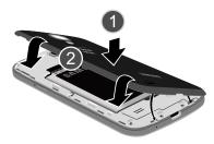
Press down along the edge of the back cover (3) until you have a secure seal.
