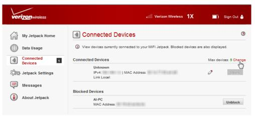
The Jetpack Settings Wi-Fi page opens. Select the number of devices from the Maximum Wi-Fi connected devices dropdown menu.
