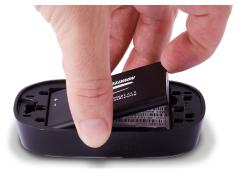
2 Align the gold-colored contacts on the battery with the gold-colored contacts on the Jetpack and gently slide the battery into place.
