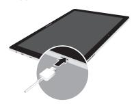
Connect the USB cable to the charging head, and then plug the charging head into a standard outlet. Unplug the charging head from the outlet and remove the USB cable from the device when charging is complete.
