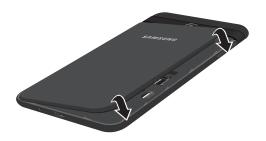
Press along the edge of the back cover until you have a secure seal.
